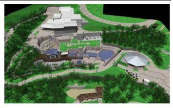
support staff. CWC work included providing the CIP concrete structural frame for the enclosure buildings and the concrete pools, tanks and perimeter walls for the exhibit area and adjacent facilities. Architectural finishes are by others. Scope of work consists of 14,000 sq. ft. of supported structural area, 53,000 sq. ft. of perimeter wall area, plus various tanks and pools.
